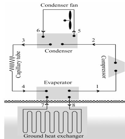
Fig.1: A schematic diagram of the system components.
