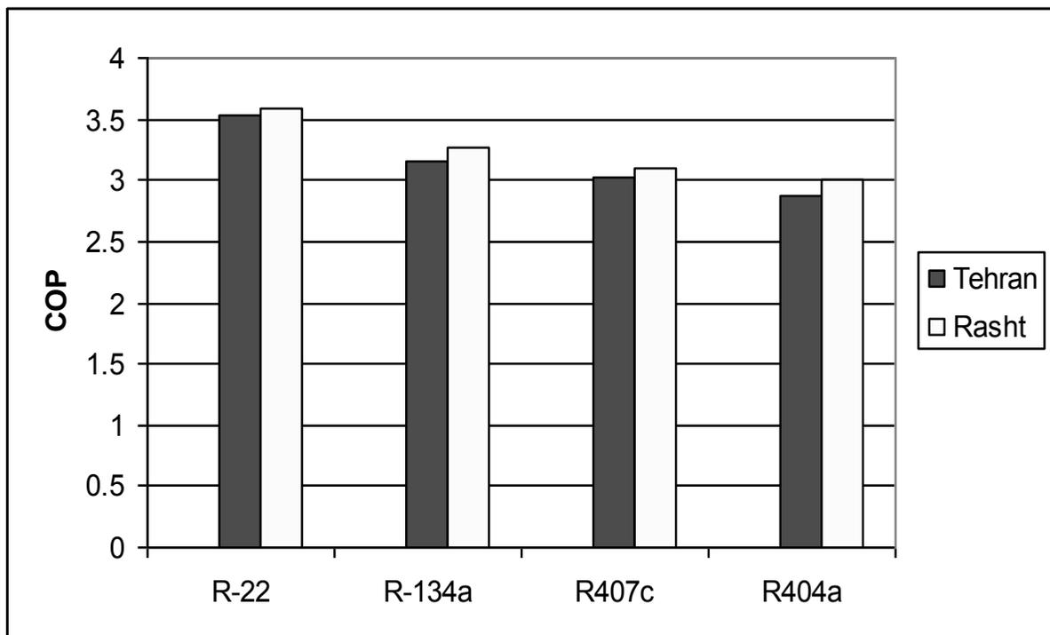
Fig.3: Energy efficiency with different refrigerants.
