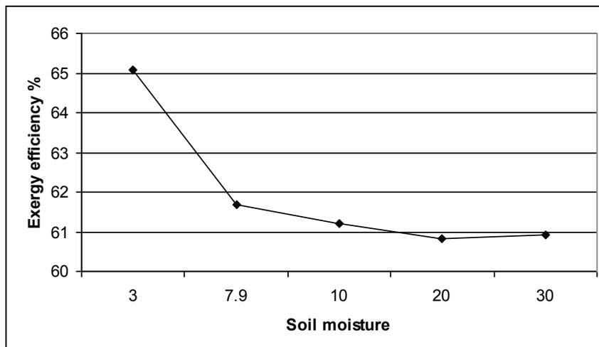
Fig.8: Effect of soil moisture in exergy efficiency (1<sup>st</sup> January).
