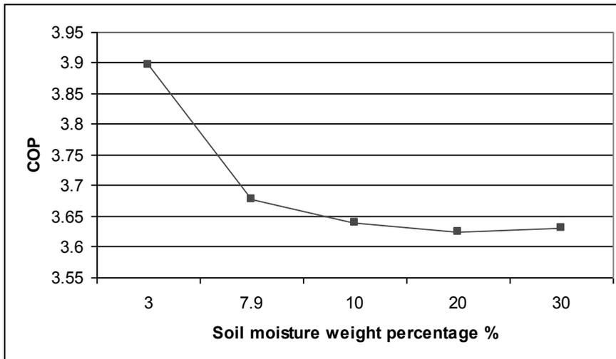
Fig.7: Effect of soil moisture in energy efficiency (1<sup>st</sup> January).
