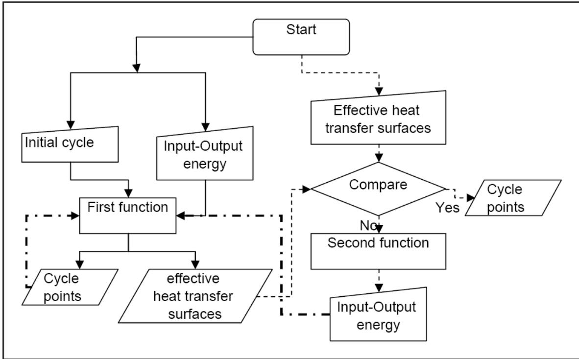
Fig.2: The flowchart of the simulation process
