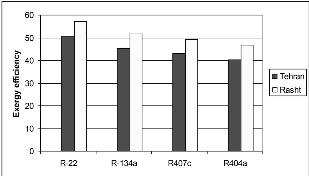
Fig.4: exergy efficiency with different refrigerants
