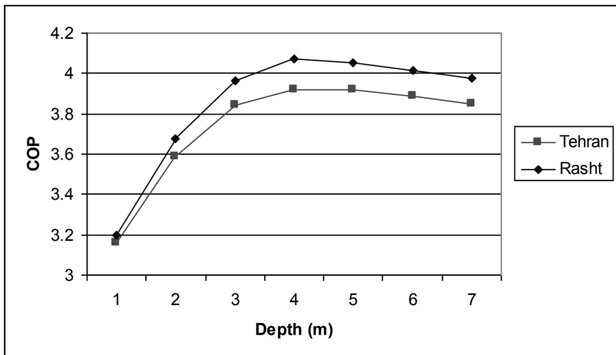
Fig.5: Energy efficiency in different depths (1<sup>st</sup> January).
