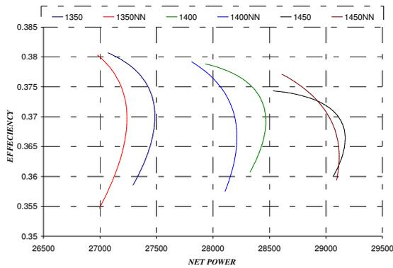
Fig.6: Variation of efficiency and power of CGAM with CPR for simulator and MFNN (NN) at  $\sigma = 0.4$
