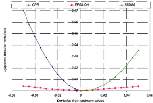
Fig.22: Effect of change in decision variables on Lyapanov function around the thermodynamic optimum condition
