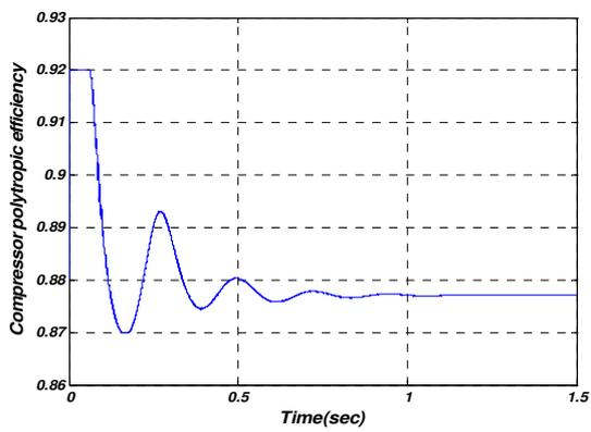
Fig.11: Computer simulated trajectory for compressor polytropic efficiency
