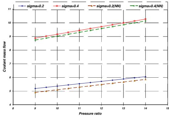
Fig.7: Variation of coolant mass flow versus CPR for simulator and MFNN (NN) at  $\sigma = 0.4, 0.2$
