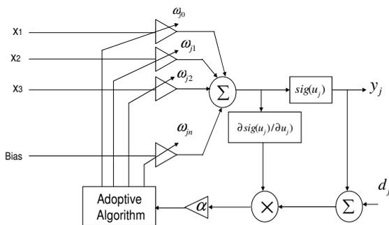
Fig.2: Implementation of BP algorithm for the single neuron located in the output layer
