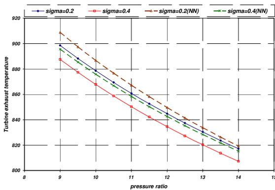
Fig.8: Variation of turbine exhaust temperature versus CPR for simulator and MFNN (NN) at  $\sigma = 0.4, 0.2$
