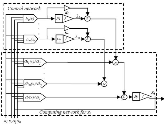
Fig. 4: Block diagram of a network for nonlinear optimization problems with equality constraints based on augmented Lagrange multiplier method
