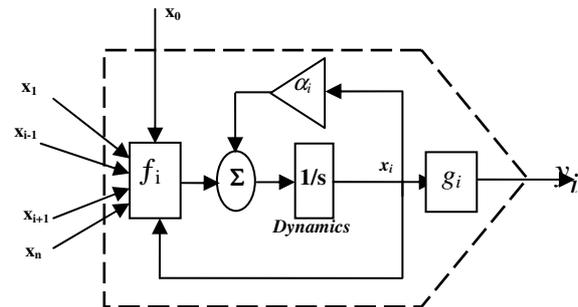
Fig.3: Schematic representation of the  $i$ th DNU
