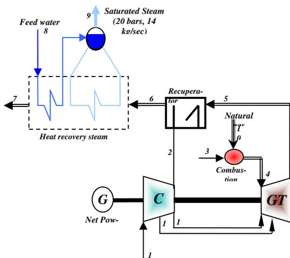
Fig.1: Flow diagram of the CGAM problem
