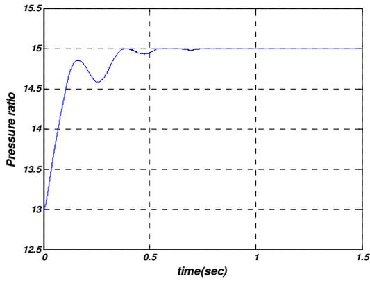
Fig.9: Computer simulated trajectory for pressure ratio
