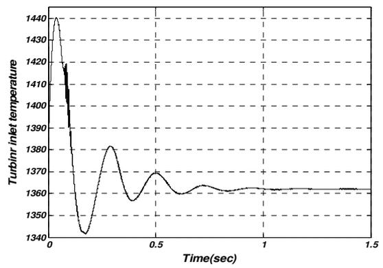
Fig.14: Computer simulated trajectory for turbine inlet temperature
