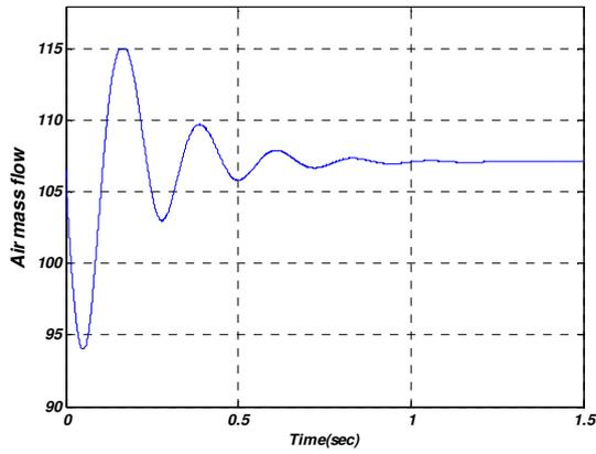
Fig.10: Computer simulated trajectory for air mass flow
