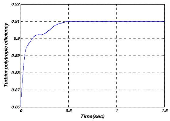
Fig.12: Computer simulated trajectory for turbine polytropic efficiency
