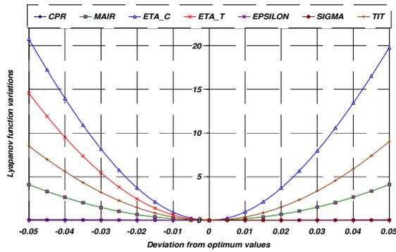
Fig.21: Effect of change in decision variables on Lyapanov function around the thermodynamic optimum condition
