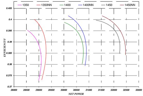
Fig.5: Variation of efficiency and power of CGAM with CPR for simulator and MFNN (NN) at  $\sigma = 0.2$
