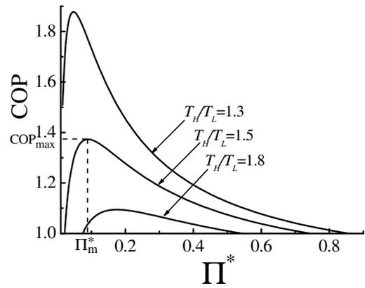
Fig.3: Influence of  $T_H/T_L$  on the  $COP$  versus the dimensionless heating load  $\Pi^*$  curves
