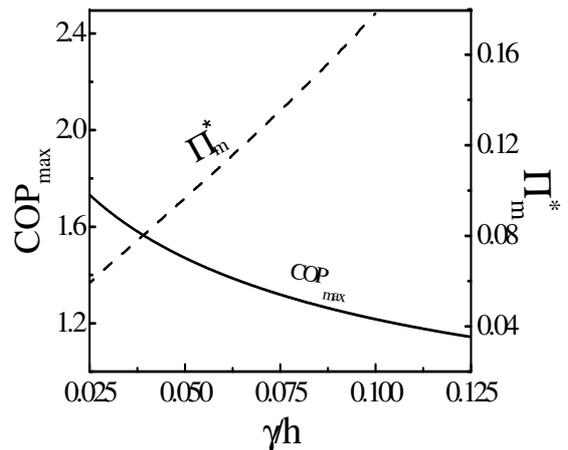
Fig.4: The maximum  $COP$  and the corresponding dimensionless heating load  $\Pi_m^*$  versus the heat leak parameter  $\gamma/h$  curves
