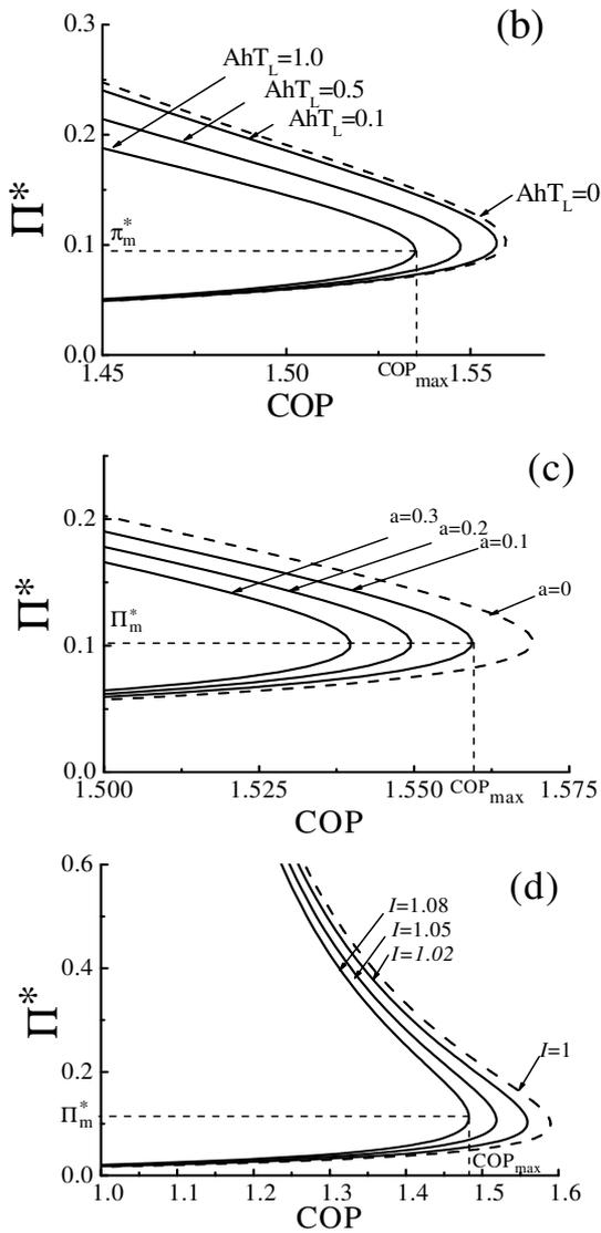
Fig.2: The influences of  $\gamma/h$  (a);  $AhT_L$  (b);  $a$  (c);  $I$  (d) on the dimensionless heating load  $\Pi^*$  versus the  $COP$  curves
