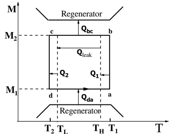
Fig.1:  $M$ - $T$  diagram of the irreversible ferromagnetic Stirling heat pump cycle.
