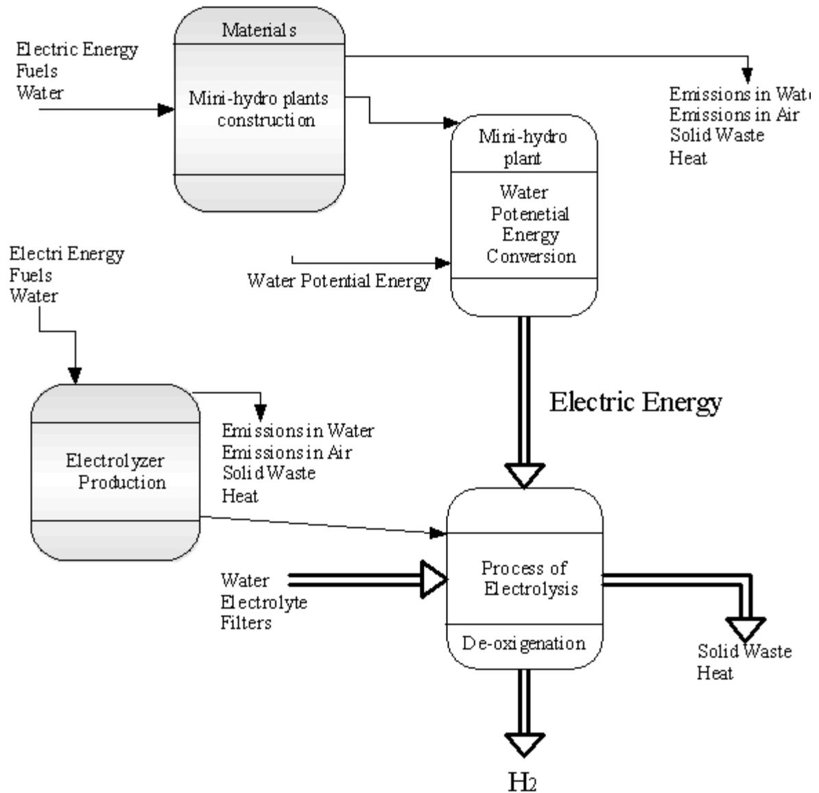
Fig. 3: Flow diagram and system boundaries of Mini-hydroelectric productive cycle.
